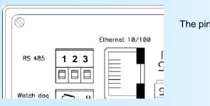
The pin (3) is Not connected
